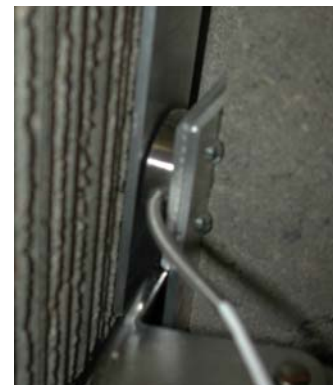
Figure 2: In Place Load Cell
