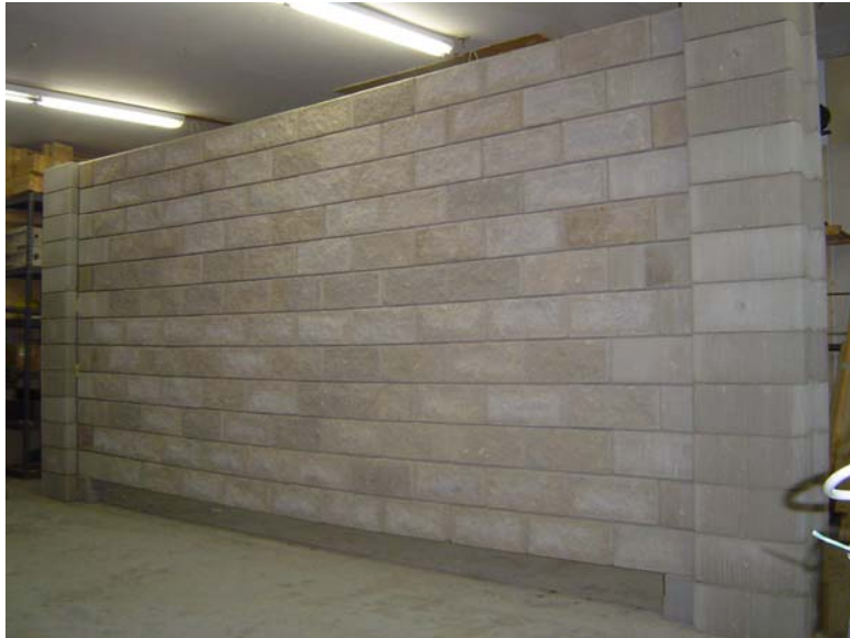
Figure 1: 11-Panel block long by 12-course tall test panel
