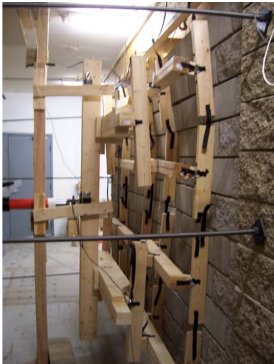
Photo A5: Spreader Frame Assembly and Block Flexing During Stressing
