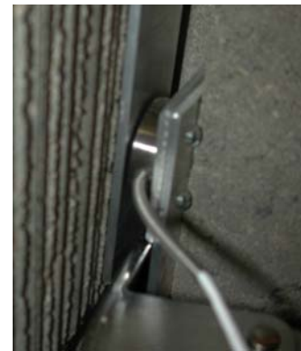
Figure 3: In Place Load Cell
